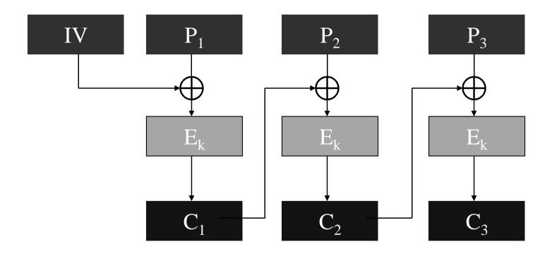
Previous *ciphertext* is XORed with current *plaintext* before encrypting current block.
